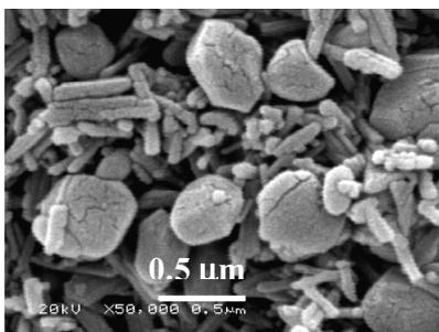
Figure 1. SEM image of the surface of titanate film deposited onto glass-FTO.
