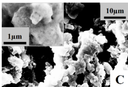
Figure 1: SEM-micrograph of a porous calcium-birnessite electrode.
