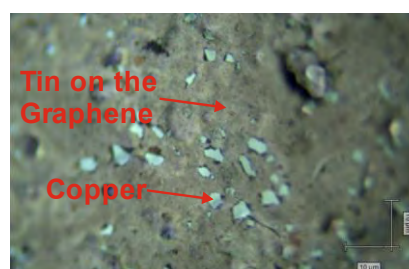
Fig. 2. The selective deposition of tin only on the not damaged graphene layer
