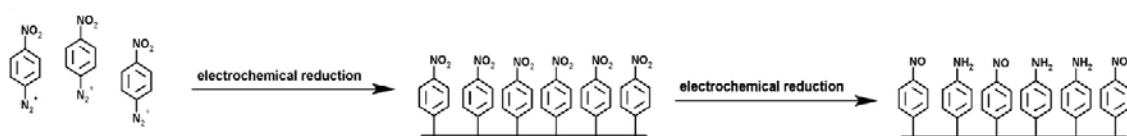
Fig.1. The schematic representation of a two-step process of the formation of a monolayer.
