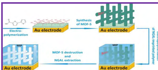
Scheme 1. Formation of NGAL-imprinted porous polymer films with help of sacrificial metal-organic frameworks.
