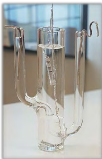
Fig. 1. Traditional macroscopic ITIES cell.
