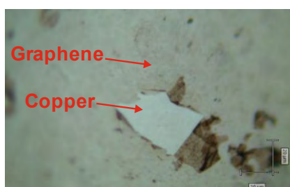
Fig. 1. The damaged layer of CVD graphene by the evolution of hydrogen
