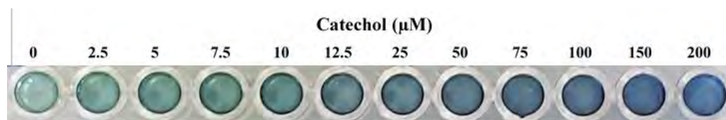
Fig. 1. Colour change of the Tyr/poly(ANI-co-AA) sensor in the presence of catechol in 0.1 M PB pH 5.0
